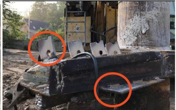
Figure 4. Discharge capability along the auger flights to convey grout to mixing zone.
