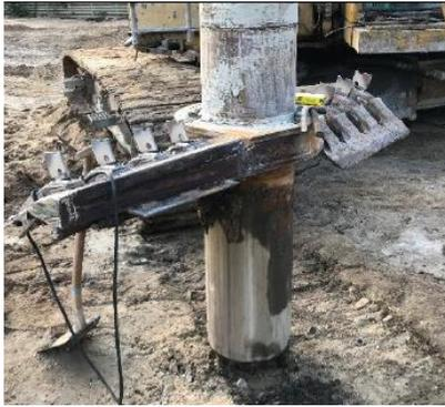
Figure 2, Mixing head with one level of flights designed to mix the soil in situ.
