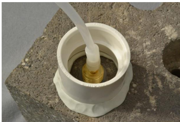
Figure 8. Water dam used for leak detection
