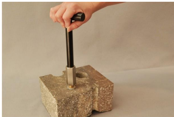
Figure 9. Removing the FLX-VP™ VAPOR PIN® sampling device
