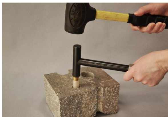
Figure 2. Installing the FLX-VP™ VAPOR PIN® sampling device
