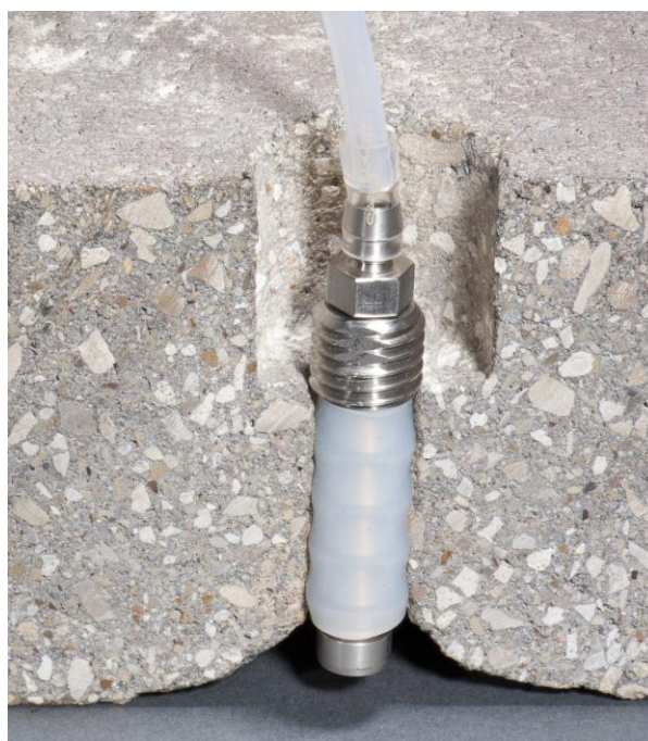
Figure 5. FLX-VP™ VAPOR PIN® sampling device sample connection
