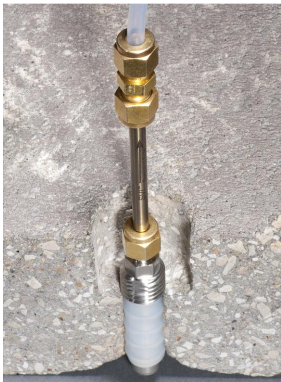
Figure 7. FLX-VP™ VAPOR PIN® sampling device with TO-17 Sorbent tube connection
