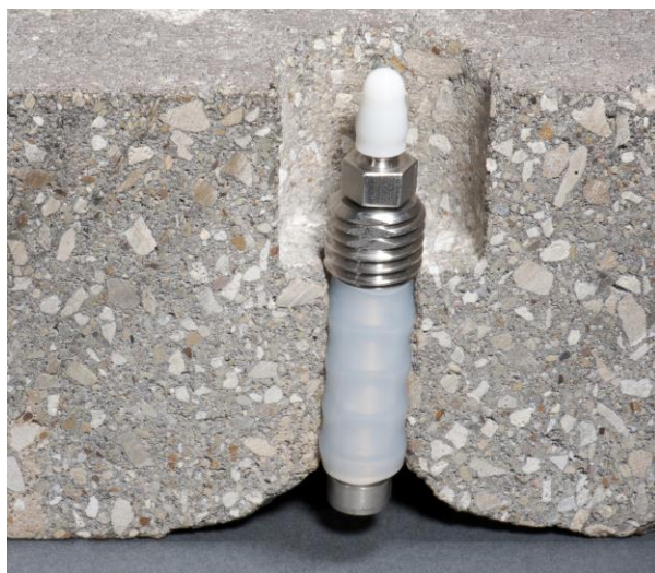
Figure 3. Installed FLX-VP™ VAPOR PIN® sampling device
